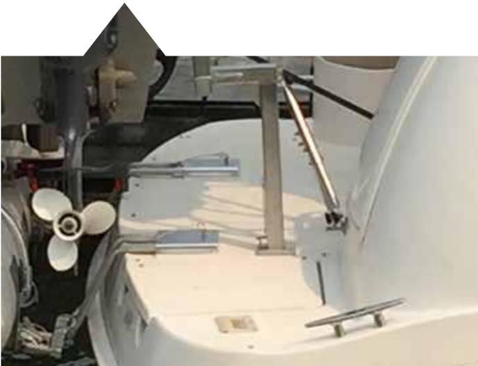
For boaters who want the opportunity to have a swim platform and stern completely clear of their davit system, Sea Wise Marine offers a removable system. By releasing the locking pin on each davit bracket, you can easily slide out the mounting arms and store for future use. Additionally, the tower is easily removed by loosening the bolting mechanism.
