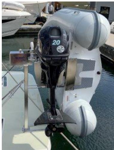
The **SeaWise** manual davit system is a complete, lightweight ready-to-install unit. It comes with a comprehensive installation manual and like all our products is backed by a 5-year limited warranty and toll-free technical support. Thanks to its geared hand-cranked mechanism, one person can easily launch or retrieve the dinghy.
